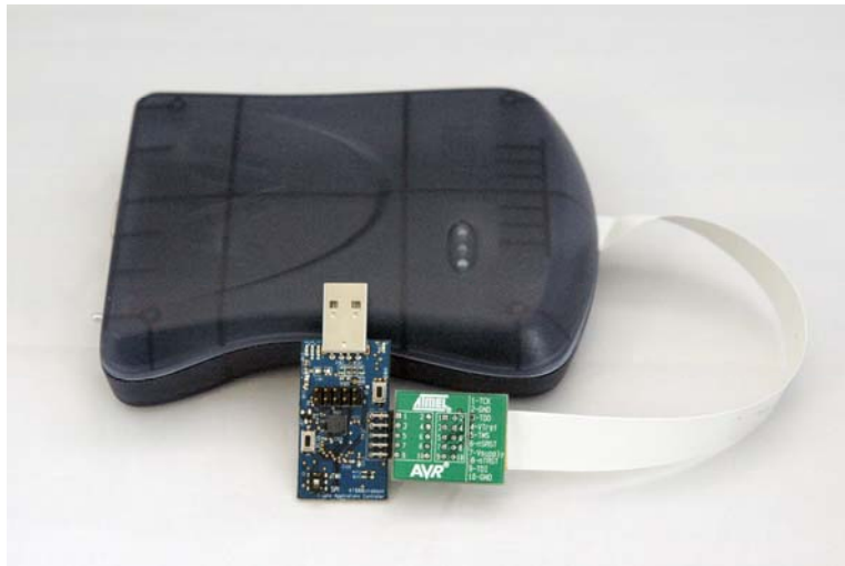
Figure 20. Connecting AVR JTAGICE mkII to the AT88Microbase
